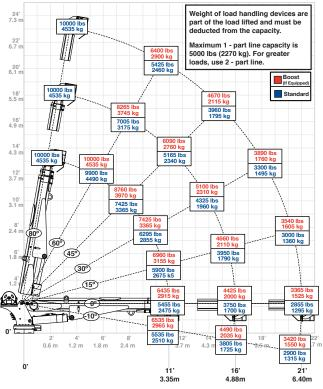
Weight of load handling devices are part of the load lifted and must be deducted from the capacity. Maximum 1 - part line capacity is 6000 lbs. (2720 kg). For greater loads, use 2 - part line.
