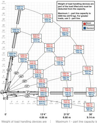
Weight of load handling devices are part of the load lifted and must be deducted from the capacity. Maximum 1 - part line capacity is 6000 lbs. (2720 kg). For greater loads, use 2 - part line.
