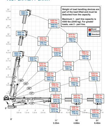
Weight of load handling devices are part of the load lifted and must be deducted from the capacity.
