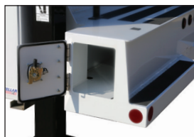
Full width longbar storage compartment integrated into the rear workbench bumper. Removable vise pedestal is standard.
