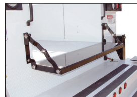
12-gauge double panel tailgate with hinged arm brackets to provide a stout working surface.
